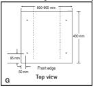
Position the base into the recess with its front edge as far forward as the adjoining plinth line will allow.
